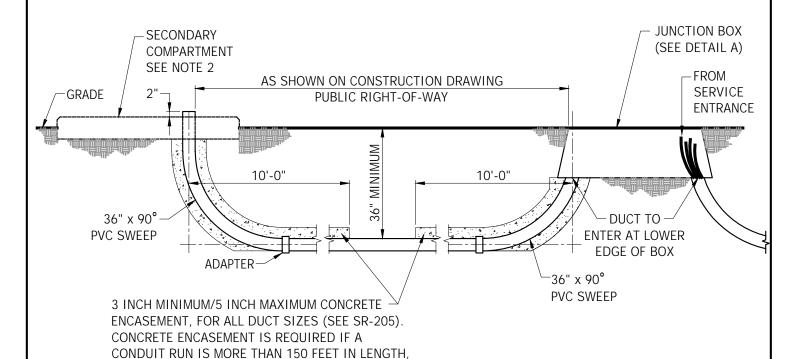
THESE REQUIREMENTS APPLY TO COMMERCIAL AND INDUSTRIAL CUSTOMERS WHO WILL BE SERVED UNDERGROUND FROM AN UNDERGROUND SYSTEM WITH THREE-PHASE SERVICE ENTRANCE EQUIPMENT RATED 600A OR LESS AND 480V OR LESS LOCATED SUCH THAT THE CUSTOMER'S SERVICE CONDUCTORS MUST CROSS PUBLIC RIGHT-OF-WAY.
