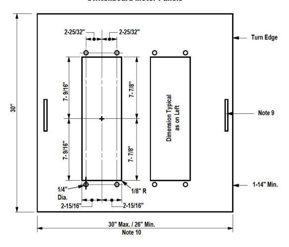
Figure 3 - Customers with Totalized Metering
