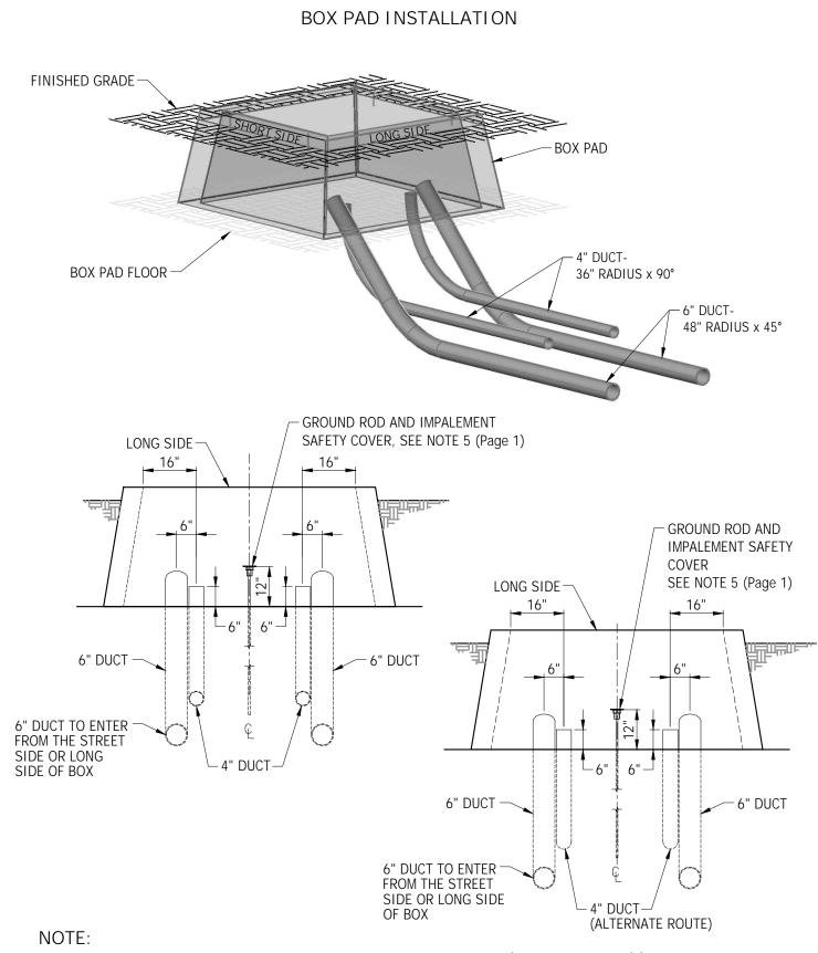
DUCT SHOWN FOR REFERENCE ONLY. FOR EXACT LOCATION AND DUCT SIZE (INCLUDING SWEEP(S) FOR FUTURE DUCT), SEE CONSTRUCTION DRAWING PREPARED BY DESIGN SERVICES. SWEEPS FOR FUTURE DUCT ARE TO BE EXTENDED ONE FOOT BEYOND THEIR CONCRETE ENCASEMENT FOR FUTURE ATTACHMENT.
