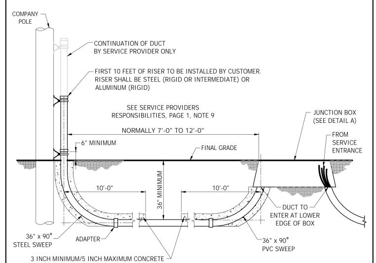
ENCASEMENT, FOR ALL DUCT SIZES (SEE SR-205). CONCRETE ENCASEMENT IS REQUIRED IF A CONDUIT RUN IS MORE THAN 150 FEET IN LENGTH, OR ANY LENGTH WITH A COMBINATION OF 270° (OR MORE) OF BENDS, NOT TO EXCEED 360°.
