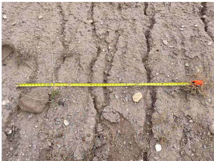
Photo 24 Closeup and scale of typical erosion rills along downhill side of bench
