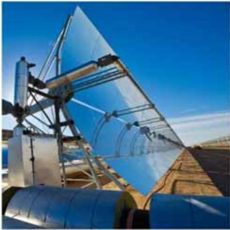
Parabolic Trough Collector
