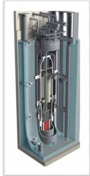
Figure 31 - NuScale Cross-section of Typical NuScale Reactor Building
