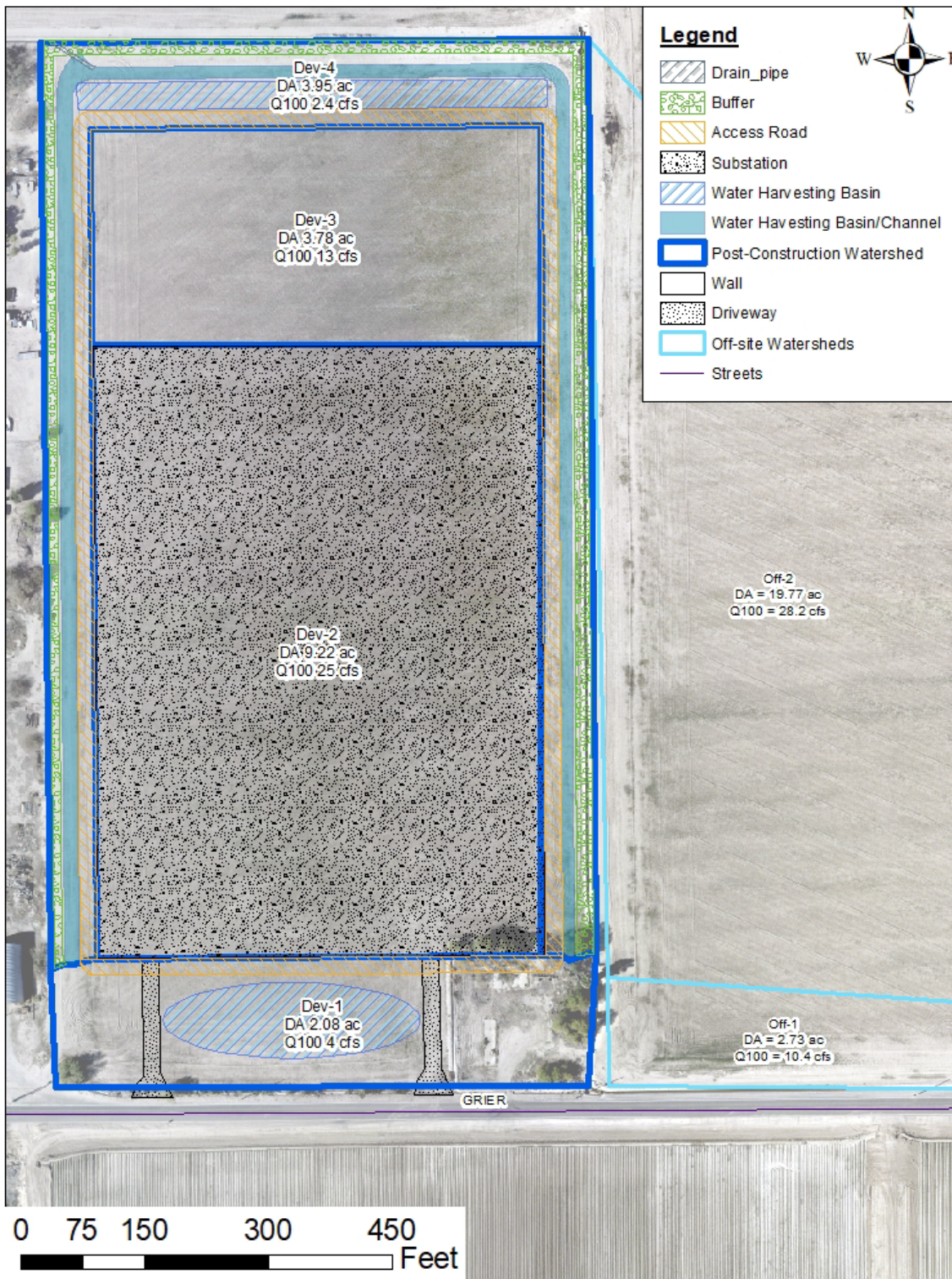
Exhibit 21. Drainage Concept with Contributing Area
